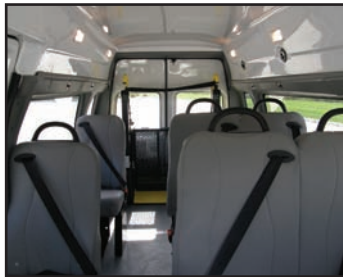
11 Passenger Seating with 2 Wheelchair Positions
